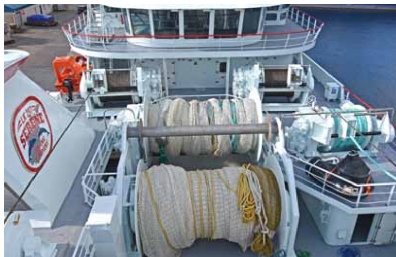
▲ Two 111t net drums are positioned across the vessel's centreline in a low waterfall arrangement.
