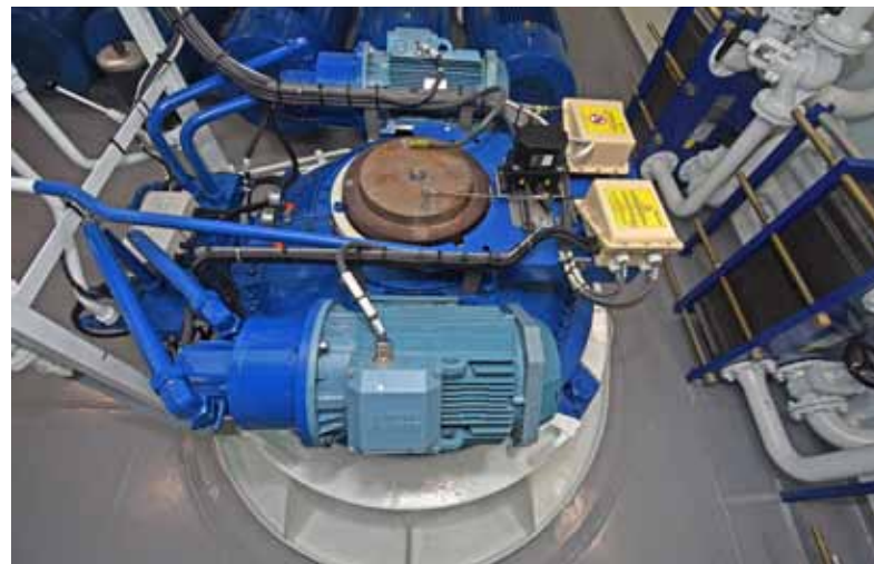
▲ Rolls-Royce Tenfjord steering gear.
