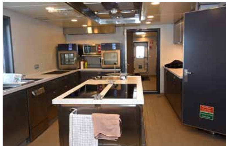
▲ ... and galley, with a double induction hob and deep-fat fryer, flush-mounted in an island unit.
