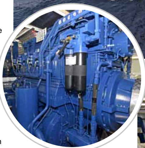
▲ Scana Volda two-speed gearbox.
