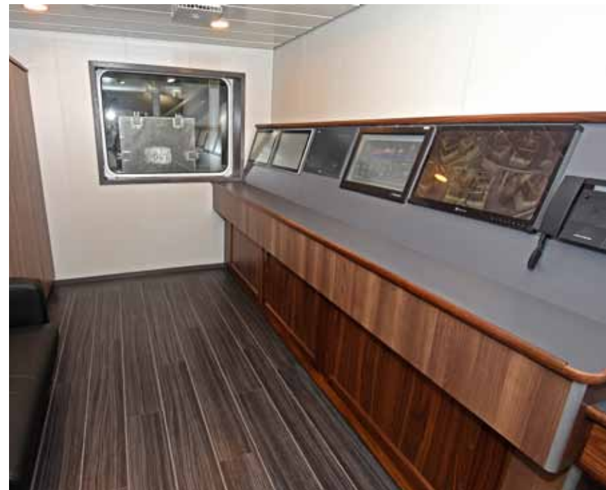
▲ The main fish-pumping control room forward in the accommodation casing looks out over the tank tops on the shelterdeck.
