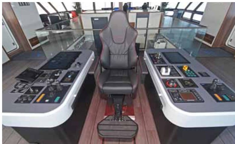
▲ Midwater trawling operations are controlled from the fishing console.
