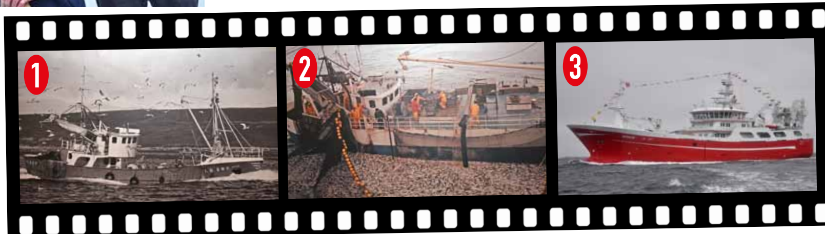
1: The 86ft open-decked purse-seiner Serene, built in 1969 at Flekkefjord... 2: ... pumping a good shot of herring on the second Serene after it was shelterdecked. 3: The previous Serene arriving in 2009.
