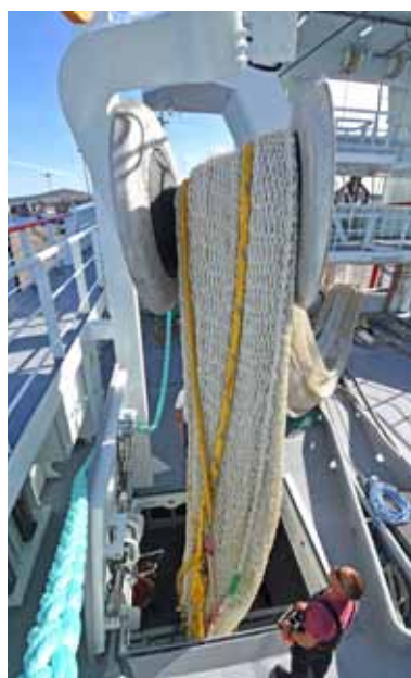
▲ Lowering one of the two 80m brailliers, supplied by KT Nets, down into the net store on the shelterdeck.
