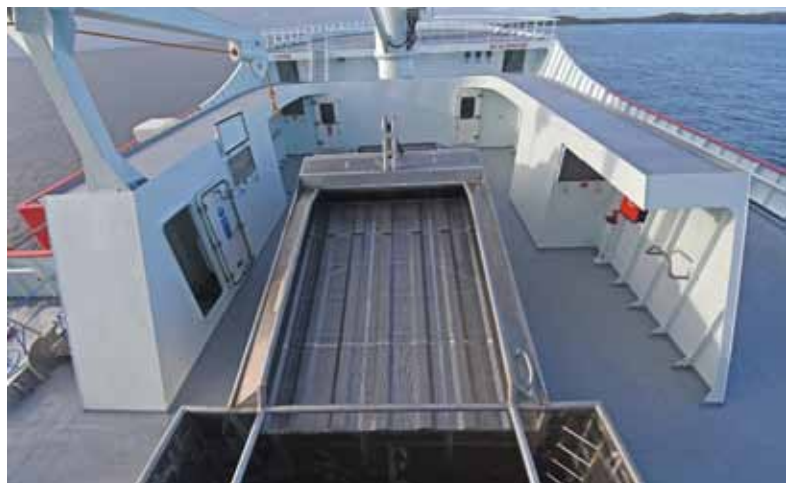
▲ The fish/seawater separator on the boat deck amidships is enclosed on three sides...
