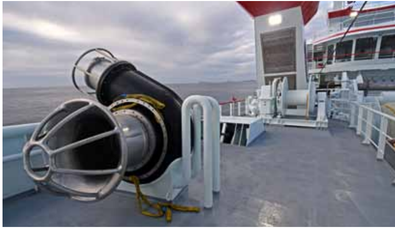
▲ SeaQuest 24in fish pump ready for action on the upper boat deck, aft of the tail-end winch...
