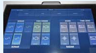
▲ Three 24in touch-screen controllers have various presets, enabling the operator to quickly select preferred displays in relation to Serene's prevailing mode of operation.
