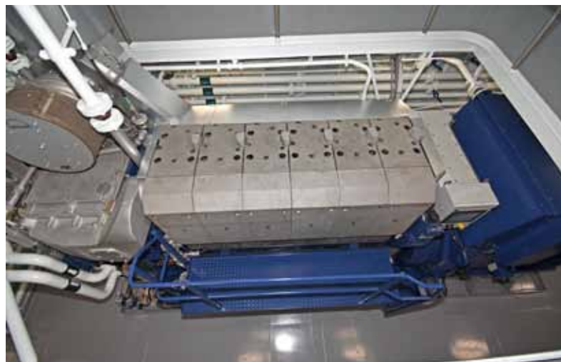
▲ MAN 6L21/31 auxiliary engines drive 1,254kW Stamford 415/3/50 generators.
