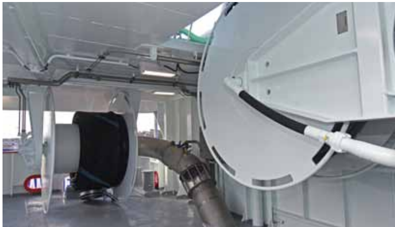
▲ ... directly above the storage reels for the fish hose and hydraulic pipes.
