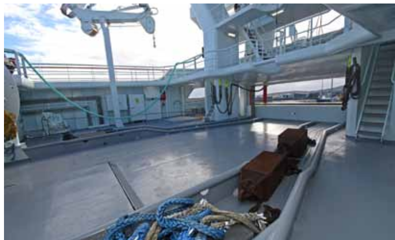
▲ The expansive boat deck trawl area is further protected by a vertical door at the transom shooting/hauling opening.
